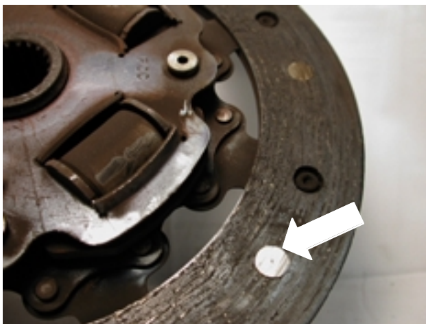
Worn Out Disc - Facing Worn Down To Rivets
