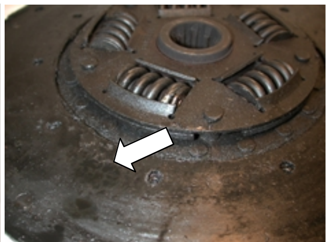
Oil / Grease Contaminated
